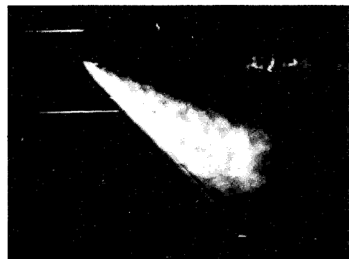
Fig. 13 Flow visualization of an aspect ratio 4.01 delta wing at an angle of attack of 20 deg and nominal acceleration of 26 \text{ft/s}^2 .
